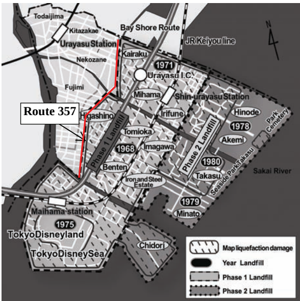
Fig.1(b) Liquefaction Warning Hazard Map in Urayasu city (Damaged area indicated by the hatched portion)
