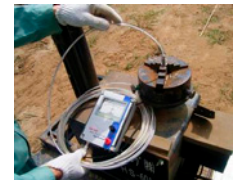
Photo 2 AC sensor with a small diameter cable
